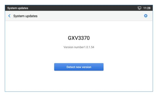
Figure 7: GXV3370 Upgrade – Detect New Version
